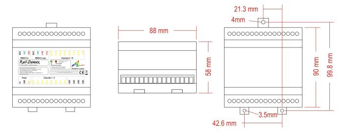
To use the surface mount option push the three bottom tabs out until they click into place. We recommend using an M4 Pan head screw.
