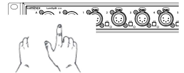
Step 2: Press the output button corresponding to the desired mode. A list of the different modes can be found on the label on the rear of the device.
