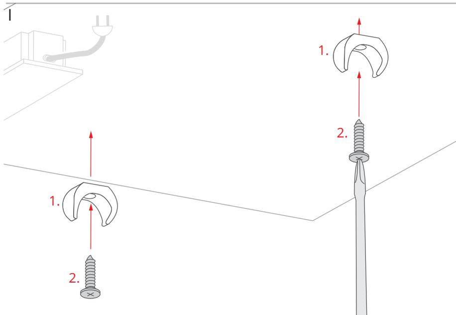
Screw the mounting brackets PLD-10 (1) to the surface with bolts (2).
