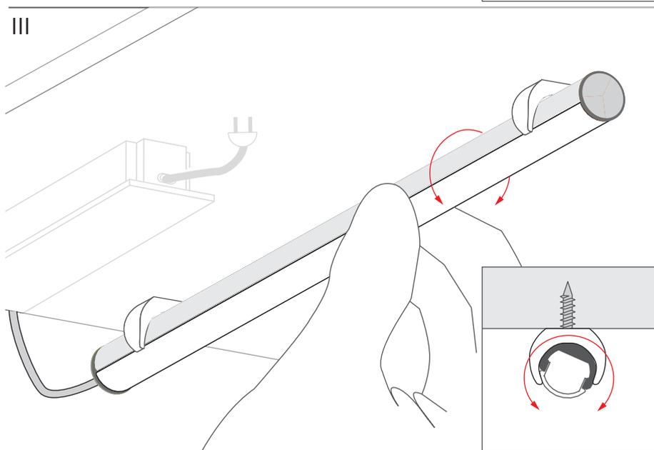
The lighting fixture can be rotated in the mounting brackets.
