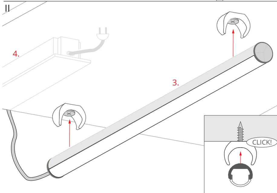
Connect the lighting fixture (3) to the 12 V / 24 V power supply (4) and mount it in the mounting brackets.
