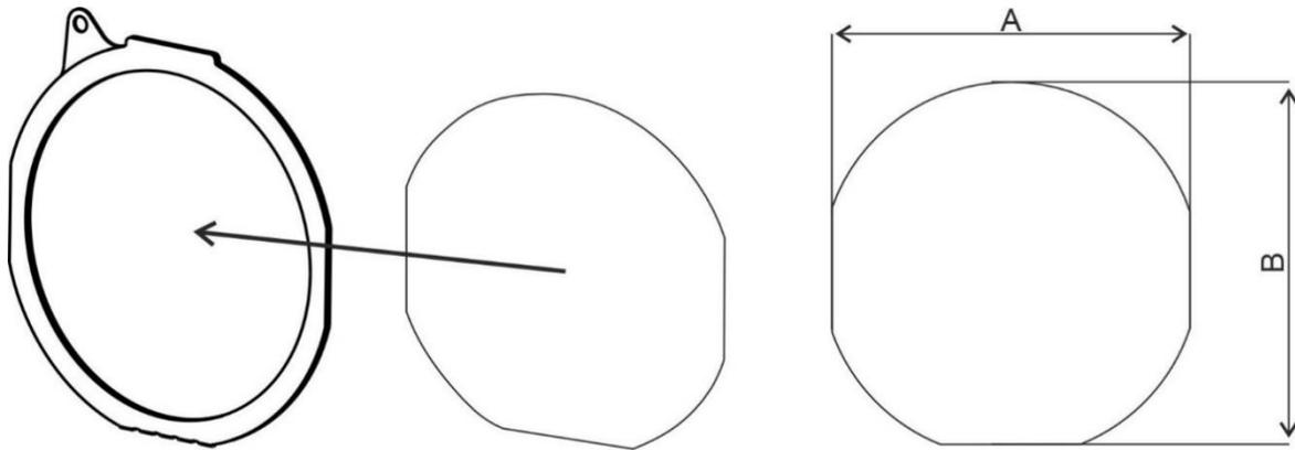
Widen slightly the Gel Holder and insert the Gel by sliding it
