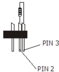
Place a 120  $\Omega$  resistor between pin 2 and 3 of a male XRL connector;
