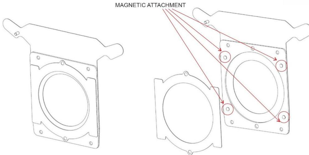
INSERT THE GOBO OR FROST IN THE APPROPRIATE SEAT AND CLOSE THE MECHANICS
