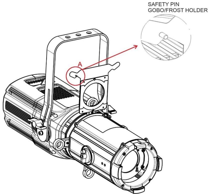
INSERT THE GOBO/FROST IN THE APPROPRIATE SLOT
