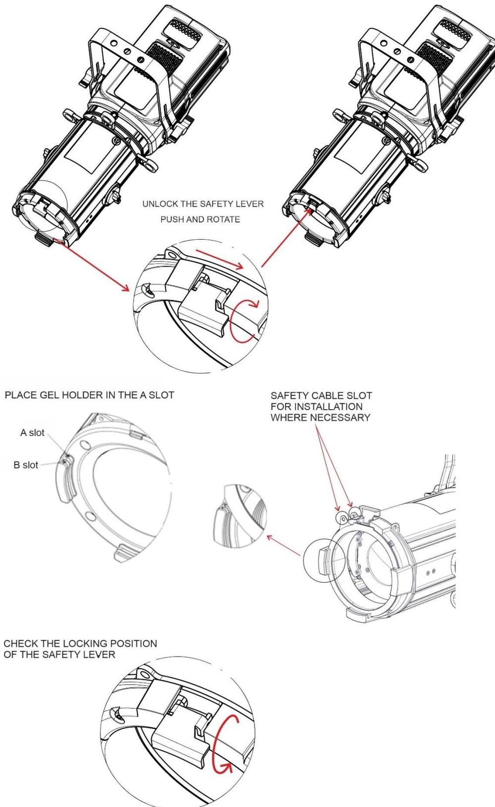
The gel holder must be inserted in position A.
