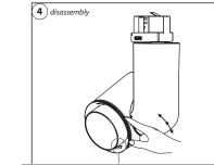
Removing the barndoor: rotate the accessory holder fully to the right or left, until you are not able to rotate it any further. (See step 5)
