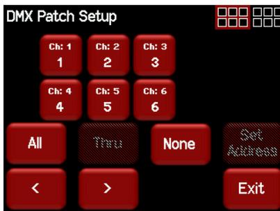
The menu shows the first 6 channels. Use the [**<**] or [**>**] buttons to see the other groups of 6 channels (if fitted). Touch a channel to select it. You can select multiple channels. To select a range of channels select your first channel then press [**Thru**] then your last channel. Use [**All**] to select all channels. Press [**None**] to de-select all channels. Selected channels turn grey. When you have selected your channel(s) press [**Set Address**].
