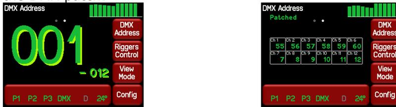
"DMX Address" with 1 to 1 Patch. "DMX Address" with Individual Patches.
