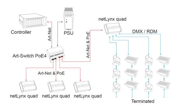
In this example, four netLynx quad products are powered using PoE supplied by an Art-Switch POE4. Each netLynx quad can convert up to 4 Universes of data.
