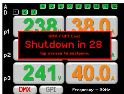
You can postpone the switch off and restart the countdown timer by tapping the screen. To disable the automatic switch off, set the time to "Infinite".
