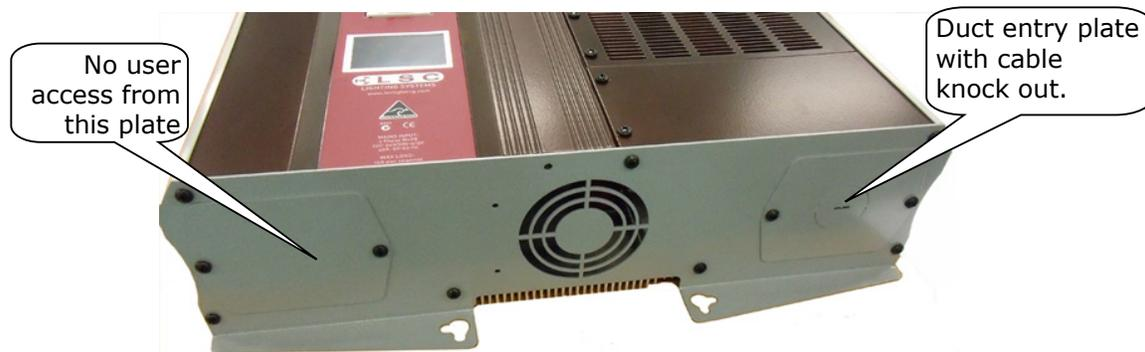
The bottom plate is provided with a cable knock-out entry. To remove the knock-out insert a flat blade screwdriver in the slot provided and twist out the metal disk and fit a M32 cable gland.
