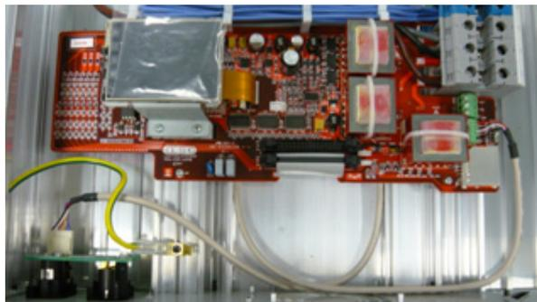
Internal wiring and cable routing. Left hand cover panel removed to show cable routing. Leave in place to avoid damage to static sensitive control electronics.
